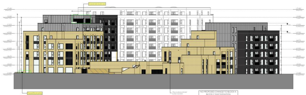
Figure 2: East Elevation indicating proposed louvres for Retail plant at Level 6 of Block B.
