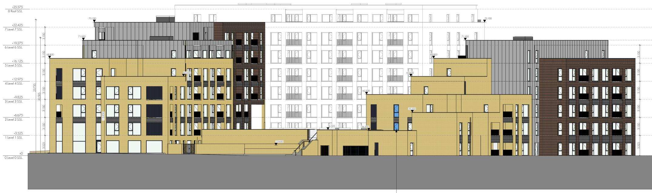
East Elevation 1:200 \_ Obscure glazing indicated by blue cross-hatch
